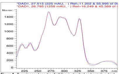
Figure 6 : Superimposed spectra of nitidine in standard and sample extract.
